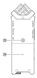
Tripod attachment screw-hole (1/4 inch) A tripod can be attached to the DR-22WL.
