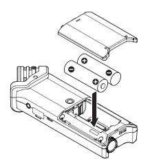
Select the same type of batteries to get an accurate reading of the remaining battery power and required minimum power for operation. (See "Battery type settings" on page 39.)
