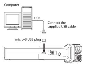
When you connect a USB cable while the unit power is on, or turn on the power after making a connection, the USB SELECT screen will pop up, prompting the user to select either to operate the unit with USB bus power or make a USB connection with the computer.
