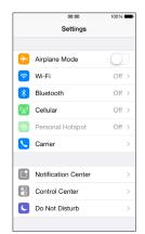
5. When Wi-Fi is enabled on for your iOS device, it will display the SSID list of Wi-Fi equipment. Select the SSID displayed on the DR-22WL.
