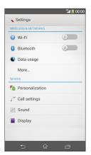
5. When you turn on Wi-Fi on an Android device, a Wi-Fi device SSID list and WPS mark will appear. Select the SSID shown on the display of the unit.
