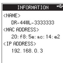
**NAME**, **MAC ADDRESS**, and **IP ADDRESS** information is shown. **NAME** shows the name to select when using DR CONTROL to operate this unit. **MAC ADDRESS** shows the MAC address assigned to the unit. The **IP ADDRESS** which is assigned by the Wi-Fi router, is a number used on the Wi-Fi network.
