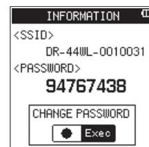
**SSID** and **PASSWORD** information appears. The **SSID** is used to identify this unit on the Wi-Fi network. The **PASSWORD** is necessary when connecting to this unit by Wi-Fi.
