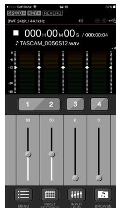
On the "INPUT SETTING" screen, you can make "LINK", "DELAY", "LOW CUT" and "LEVEL CONTROL" settings. Touch the underlined item that you want to change and adjust the setting.
