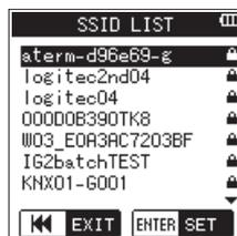
3. From the list shown on the **SSID LIST** screen, use the **wheel** to select the desired **Wi-Fi** router from the list shown on the **SSID LIST** screen, and press the **ENTER/MARK** button to set it.
