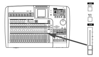
The 2488MKII sub mixer facility allows you to add up to eight more inputs (usually on mixdown) to the twentyfour tracks already recorded. These could be inputs from a multi-timbral MIDI device, synchronized using MIDI clock information from the 2488MKII driving a sequencer. The eight inputs from A through H are pressed into service here and they feed a bus that can be routed to the stereo bus (or to the recorder in bounce mix—see "Making a bounce mix" on page 58).
