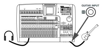
2 Play the guitar, and adjust the level using TRIM control H so that when you play a loud note, the OL indicator above the INPUT-H key lights very briefly. Then turn the TRIM counterclockwise a little to set the appropriate level.
