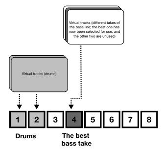
Alternatively, if you want to assemble a track for the whole song, you could assign the three different takes of the part to three different active tracks and use the track editing functions to copy and paste the good parts of each track to make a perfect whole. Then use the two non-perfect tracks with other virtual tracks for new parts.
