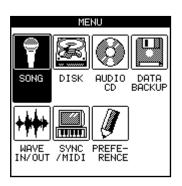
Turn the JOG/DATA dial until the DISK item is highlighted, and then press the YES/ENTER key.
