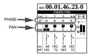
Use this screen to make pan, phase and fader setting for four channels at a time on this screen (linked channels still count as two channels here).
