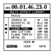
Use the **◄/►** cursor keys to select either the **PRESET** memory banks, the **USER** memory banks, or **SAVE** the current setting. The left side of the **PRESET** memory banks provides a description of the effect (**GRUNGE**, **CLEAN FUNK**, etc.).
