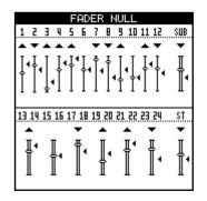
When a physical fader position and internal fader position are not matched, a  $\nabla$  or  $\triangle$  will appear above the fader icon. These triangles indicate whether a physical fader needs to be (raised  $\triangle$  or lowered  $\nabla$  to) match its internal fader position.
