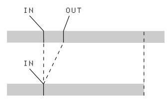
The source and destination are the same, and after the operation, the material which followed the OUT point now moved to follow the IN point. Material which was between the IN and OUT points is deleted. The result is therefore shorter than the original.
