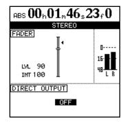
In this case, the LVL value corresponds to the physical fader level, and INT gives the internal virtual fader value (as marked by the triangular symbol beside the on-screen fader).
