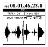
Press the SELECT key of the track that you want to view. The display changes to the waveform of that track.
