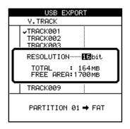
Select the final bit depth (RESOLUTION) of the exported files (16 or 24 bits). The file size of the exported data changes according to the bit depth.
