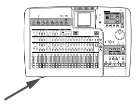
Plug in and turn on the 2488MKII. The power switch is on the rear, by the power cord.
