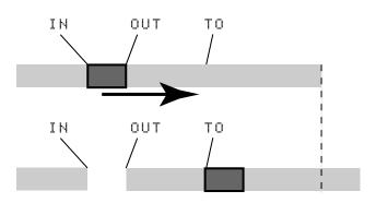
After the operation, the selected section of the source between the IN and OUT points is replaced by silence.
