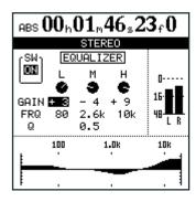
Use the cursor keys and dial to select and adjust the EQ parameters for the stereo bus. See "EQ" on page 31 for information about setting methods, etc.
