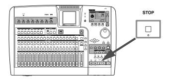
11 To return to the zero position, where your song began, press and hold the STOP key, and press the REW key (marked as RTZ—"return to zero").
