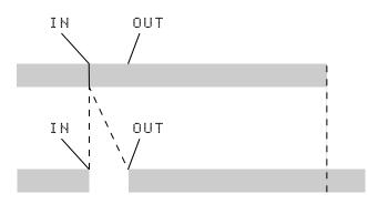
The source and destination are the same, and after the operation, the track is split at the IN point, with the material which followed the IN point now moved to follow the OUT point. The result is therefore longer than the original.
