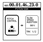
2 If the PITCH CONTROL section at the left of the screen is not active (it is not surrounded by the thicker frame), press the ◀ key to move the cursor there.
