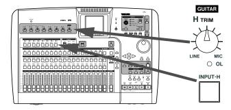
3 Press and hold the INPUT-H key so that it starts to flash. While holding it down, press the SELECT key of channel 1. Now both these keys will flash.
