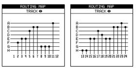
Use the left and right cursor keys to change between viewing channels 1 through 12, and 13 through 24.
