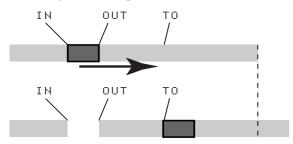
After the operation, the selected section of the source between the IN and OUT points is replaced by silence.
