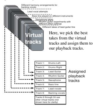
When a virtual track is assigned to be an "active" disk track, it cannot be assigned to any other track.
