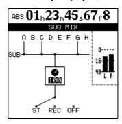
This shows the current assignment of inputs to the sub mix, and the current assignment of the sub mix output.
