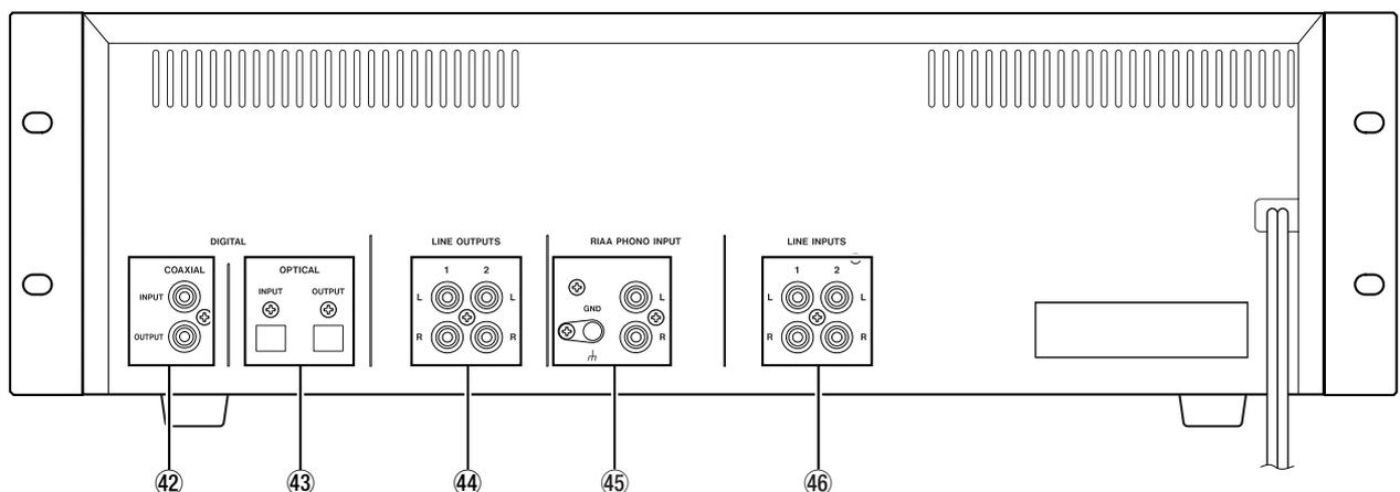
The CC-222MKII line analog inputs and outputs all operate at the  $-10\text{dBV}$  level. For details of input and
