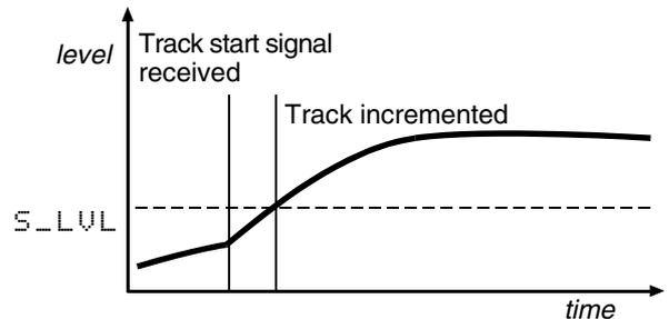
A fall and subsequent rise in volume alone when recording digitally from CD, MD or DAT is not sufficient to trigger an automatic track increment.
