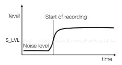
Synchronized recording stops when the sound level drops below the threshold for five seconds:
