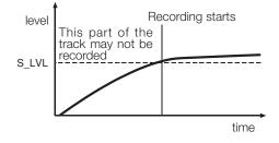
If the "noise floor" is higher than the threshold, synchronized recording will not take place.
