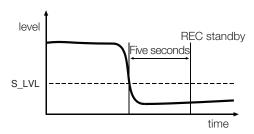
If you set the threshold value so that only high-level signals trigger recording, remember that this will not record the start of a piece which has a slow fade-in:
