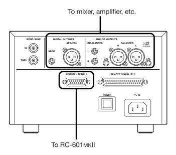
If you have the RC-601MKII remote control unit, connect the PLAYER UNIT port on the RC-601MKII rear panel to the REMOTE (SERIAL) port on the CD-601MKII rear panel using the cable supplied with the RC-601MKII.
