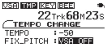
The screenshot shows the 'TEMPO CHANGE' screen. At the top, it displays 'USA TMP KEY BEE' with a mouse cursor icon. Below that is '22 Trk 68 M 23 S'. A horizontal line separates the header from the main content. Under the line, 'TEMPO : -50' is shown. Below that, 'FIX\_PITCH : VSA OFF' is displayed, with 'VSA OFF' highlighted in a dark box.
