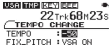
When the **TEMPO** value is set to anything other than 0, the tempo mode is **ON**, and playback follows the set tempo. **TMP** appears in inverse at the top of the screen.
