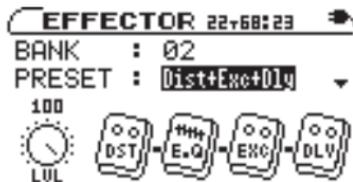
On the EFFECTOR screen, use the CURSOR (▲, ▼) keys to select items and the VALUE (+, -) keys to adjust settings in the same way as on other screens. Use the CURSOR (◀, ▶) keys to move between level knobs and effect modules.
