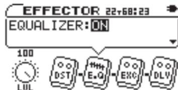
Use the **CURSOR** (▼) key to open the EQ screen where you can check and adjust the seven-band equalizer.
