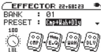
After selecting an effect bank, select an effect preset by using the down **CURSOR (▼)** key to highlight the **PRESET** value. Then use the **VALUE (+, -)** keys to select a preset. Each preset uses a different combination of effect modules. (See the “Effect preset lists” on page 41.)
