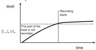
Also remember that when recording from an analog source, the threshold should be set so that it is higher than the "noise floor" (the base level of hiss, pops and crackles which may come from an older vinyl recording, for example). If the "noise floor" is higher than the threshold, a false start will occur:
