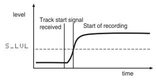
when recording from any source other than the ones described above (that is, any digital source other than DAT, CD or MD, or any analog source), recording starts when the input signal level exceeds the trigger level.
