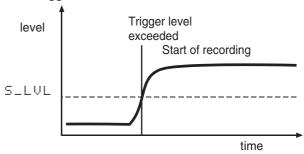
In this last case, if the signal level is already higher than the trigger level, recording starts immediately.
