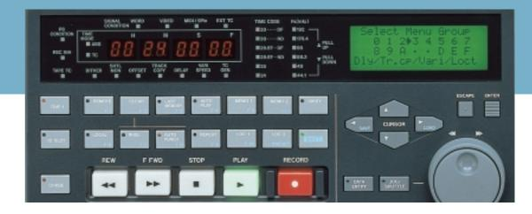
The DA-98HR's front panel combines familiar transport controls with a wide variety of dedicated buttons that ensure quick and efficient operation. A comprehensive LCD display and data/jog wheel allow fast entry of numeric values.
