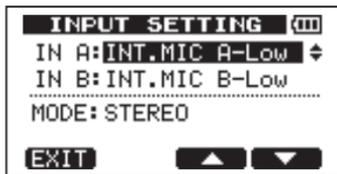
The **IN A** and **IN B** items are used to set the input sources for the **INPUT A** and **INPUT B** channels.
