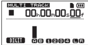
If you turn up the **MASTER LEVEL** knob and the **VOLUME** dial, you can hear the guitar on the left channel of your headphones, and the **L** meter on the screen moves.
