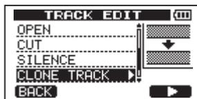
Use this function to duplicate a single track, a track pair or the master track on a different track or track pair. Each track is copied entirely, so the IN/OUT/TO points have no effect.
