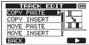
This function copies the audio data from between the IN and OUT points on the COPY source track, and pastes it on the COPY destination track starting from the TO point. This operation does not change the COPY source track.
