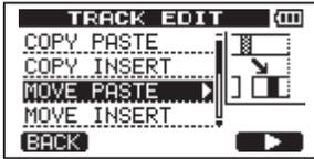
The audio data between the IN and OUT points on the MOVE source track is removed and pasted in the MOVE destination track starting from the TO point. This operation leaves a silence between the IN and OUT points on the MOVE source track.
