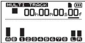
Turn up the **TRACK 1 LEVEL** and **MASTER LEVEL** knobs and the **VOLUME** dial to hear the guitar sound through headphones. When doing so, the **L** and **R** meters on the right side of the display become active.
