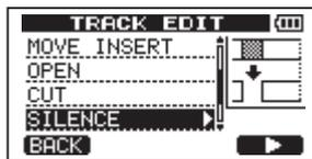
This function cuts (deletes) the audio data between the IN and OUT points on the selected track, leaving silence between the IN and OUT points, as though there had been no recording.
