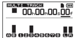
Raise the TRACK 3 LEVEL knob, MASTER LEVEL knob and VOLUME dial as necessary to hear the mic input through the headphones.
