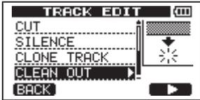
Use this function to completely erase the selected track. This erases the entire track, so the IN, OUT and TO points have no effect.
