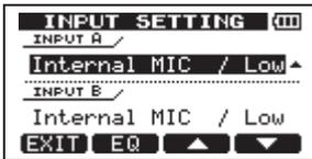
Use the INPUT A and INPUT B items to set the input sources for the INPUT A and INPUT B.
