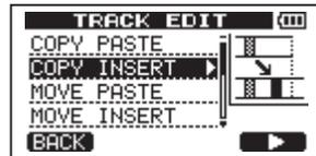
This function copies the audio data from between the IN and OUT points on the COPY source track, and inserts it on the COPY destination track starting from the TO point. This operation does not change the COPY source track.
