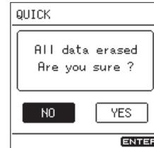
Turn the wheel to move the cursor to **YES** and press the **ENTER/MARK** button to execute the function and return to the previous screen.
