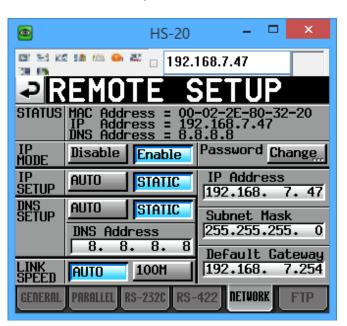
In this case the IP address was set manually (STATIC), and is 192.168.7.47
