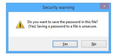
In this case, selecting YES will add the password you used to connect to your HS-20 into the VNC file. Although it says "insecure", the password is not saved in plain text, but someone with access to your computer can find the actual password by using other available tools. If the computer is on the same trusted internal network as the HS-20, this should not be a problem.
