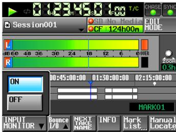
When ON, sound input through the assigned input connector is always output from this unit.
