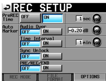
When the auto marker function is ON, marks can be added upon PREREC start/ recording start / end when audio overs occur, at regular time intervals and when synchronization errors occur (see “OPTIONS page” on page 90.)
