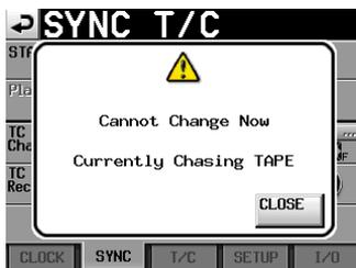
To change a setting, press the **STOP** key once to stop the transport beforehand. After making the change, press the **PLAY** or **PAUSE** key to resume emulation mode.
