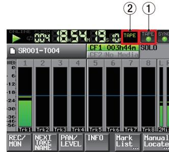
When the tape emulation function is ON, the time code display (②) is limited to one of the following three types.
