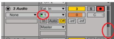
That is because the monitoring setting of the track is off and you cannot listen input sounds in this condition.
