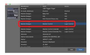
**6.** For Device: Mackie Control, set the Output Port to "Model 12 DAW Control OUT".
