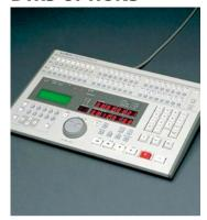
RC-898 Multi-unit Remote Controller offers centralized transport and record function control of up to 6 DTRS recorders. The RC-898 also features parallel and RS-422 (SONY P2 protocol) ports which allow the RC-898 to control an external ATR or VTR including Jog shuttle operation
