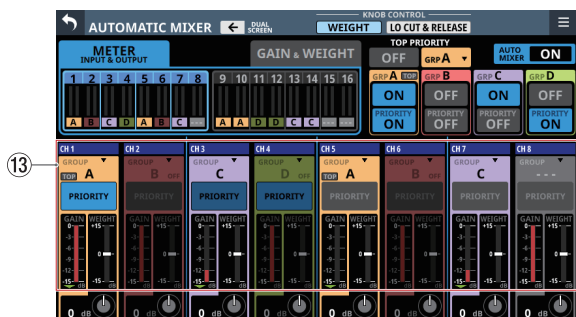
AUTOMATIC MIXER Screen when LCD knobs are controlling WEIGHT
