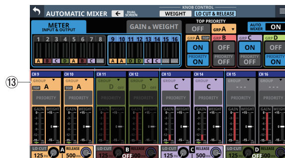
AUTOMATIC MIXER Screen when LCD knobs are controlling LO CUT & RELEASE
