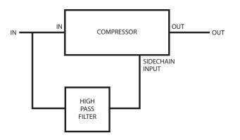
Only the sibilants pass through the highpass filter. When the input signal contains sibilant material, the output of the filter causes the compressor to compress the signal. The compressor only operates when a sibilant is present.
