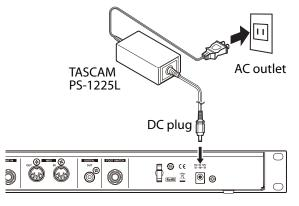
Use the hook (cord holder) on the rear panel to secure the AC adaptor cord. When connecting the cord to the unit, wrap it through the holder to prevent it from becoming disconnected during use.
