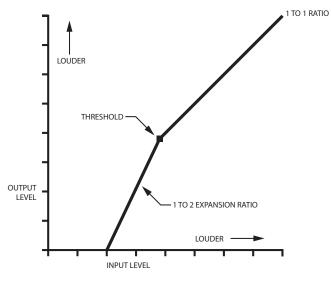
When expanders use ratios higher than 1:10, sounds below the threshold are faded out very rapidly. This effect is called gating and can sound very abrupt. Adjusting the gate ratio can smooth out the abrupt change. The graph below shows the input/output curve for a typical gate.
