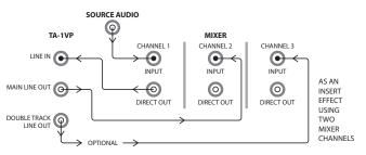
For this configuration, your mixer must provide direct channel outputs.
