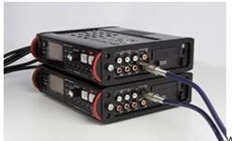
When using the cascade function, the master unit controls the REC/PAUSE start (front of unit) and the STOP and PLAY/PAUSE keys (on the top) from multiple DR-680MKII units at the same time.
