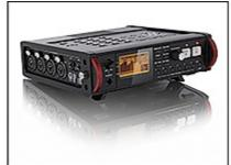
SD, SDHC and SDXC cards are used as recording and playback media, and the compact form offers excellent vibration resistance. Along with the included shoulder strap, this unit has a built-in folding stand for tabletop use, making operation easy in a variety of situations.
