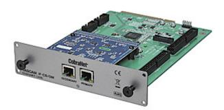
The IF-CB/DM interface card for the Tascam DM-3200 and DM-4800 digital consoles allows connection to CobraNet® audio networks over CAT-5 cable. The card transfers up to 16 channels of digital audio to and from CobraNet devices. The DM-3200 can accommodate one IF-CB/DM (Slot 1), while up to two cards can be used in the DM-4800 (Slots 1 and 3) for a total of 32 audio channels in and out. This card helps reduce cost, labor and time in live applications and when installing large-scale systems.
