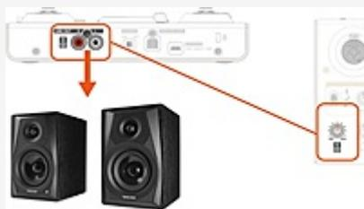
The **LINE OUT** jacks allow monitor speakers to be connected for checking video or music while it is being created. Volume can be adjusted separately from that for the headphone jacks.
