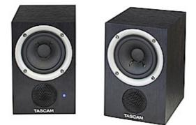
The VL-M3 is a highly compact active monitor set perfectly suited as an extension to computer systems, multi-track recorders, or any portable music player. It consists of two bass reflex enclosures with 3-inch full-range loudspeakers powered by a 24-watt amplifier built into the left cabinet. A stereo line input on RCA connectors is provided as well as binding terminals for the loudspeaker connection between the left and right cabinets.
