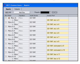
When you set the input bus, a device port is automatically selected. If necessary, you can change the device port. The device port pull-down list indicates all available input ports for the US-1641.
