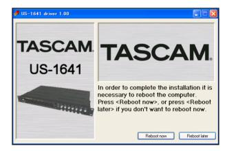
11 After the computer has restarted, select Start > Settings > Control Panel, then click TASCAM US-1641 Control Panel to open the US-1641 Control Panel. If the driver version, device name and other data appear to be correct, the installation was successful.
