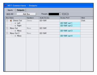
When you set the output bus, a device port is automatically selected. If necessary, you can change the device port. The device port pull-down list indicates all available output ports for the US-1641.
