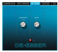
**FREQUENCY:** 1 to 4 kHz (default: 1.15 kHz) Sets the lowest frequency that the de-esser effects.
