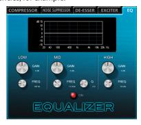
The frequency response is shown even when the equalizer is off. The equalizer has a high-shelf HIGH band, a low-shelf LOW band and a peaking (bell-shaped) MID band.
