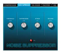
THRESHOLD: -84 to -24 dB (default: -64 dB) Sets the threshold level that will cause noise suppression if the input signal becomes less than it.
