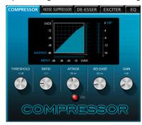
The three meters show the level of the signal input to the compressor ("INPUT"), the level of the signal output from the compressor ("OUTPUT") and the gain reduction caused by the compressor ("GR").
