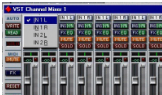
Illustration 6.06 - Input selection window, showing Mutes and Solos
