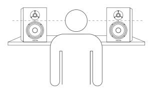
4 Recommend Place the VL-X5 horizontally. If you Placing VL-X5 horizontally, refer to the following diagram.
