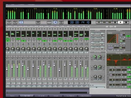
The clear mixer screen shows 24 channels at once, each with aux level meters, pan knob and faders and allows quick access to dynamics, EQ and other settings.
