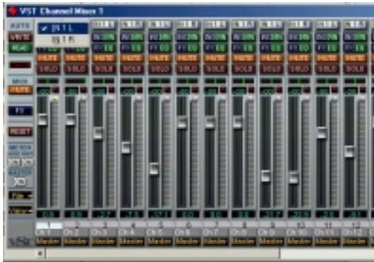
Illustration 6.06 - Input selection window, showing Mutes and Solos
