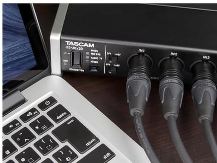
USB 3.0 is used in the US-20x20 for 24-channel transmission at 192 kHz/24-bit. This is not possible with USB 2.0.
