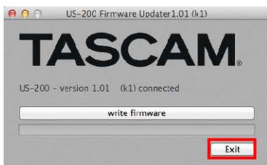
10. Reconnect the USB cable to start the unit with the new firmware.
